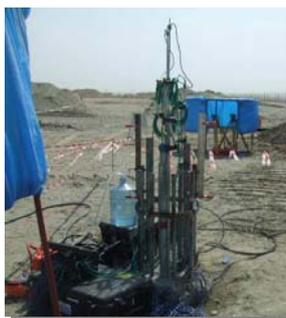
600mm pile under test
