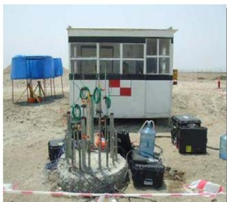
1000mm pile under test
